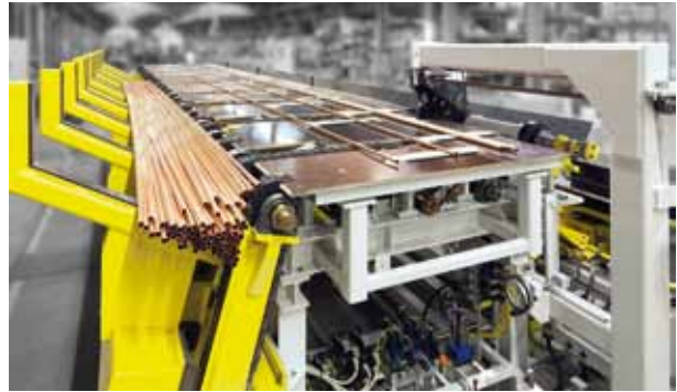
Copper tubes: straightened, tested and cut
